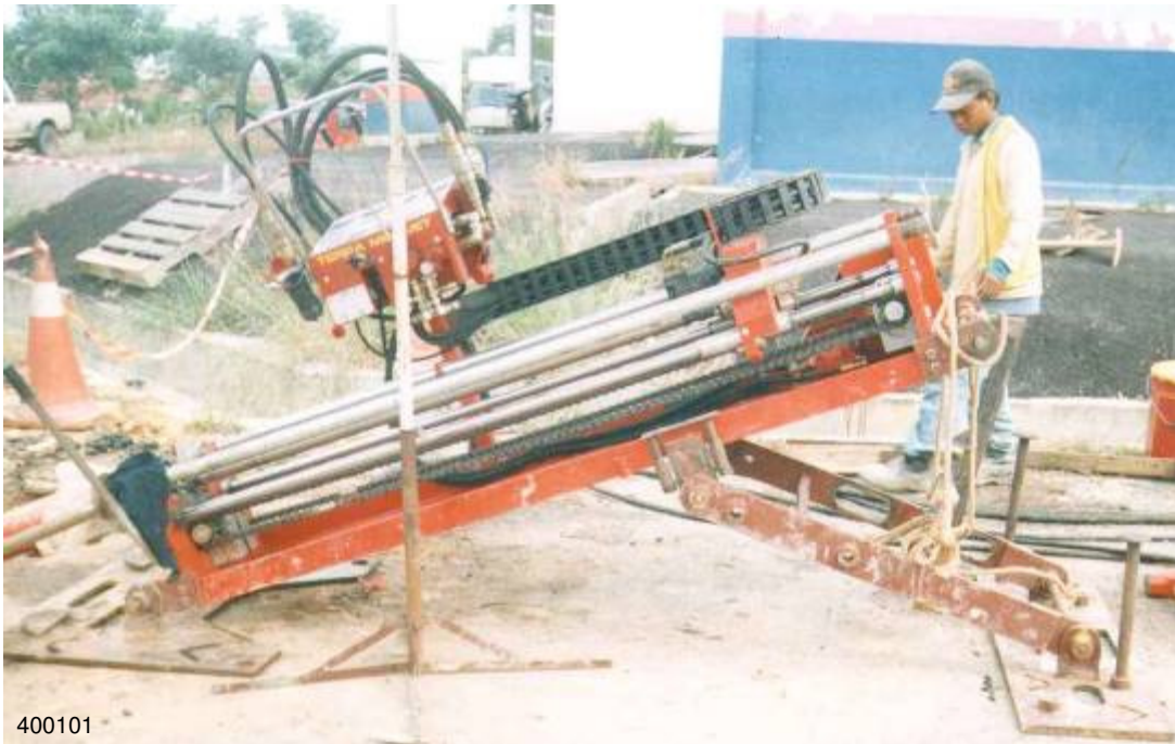
Picture left: The pit frame TERRA MINI- JET MJLV 1400 with accessories for the surface launch.
