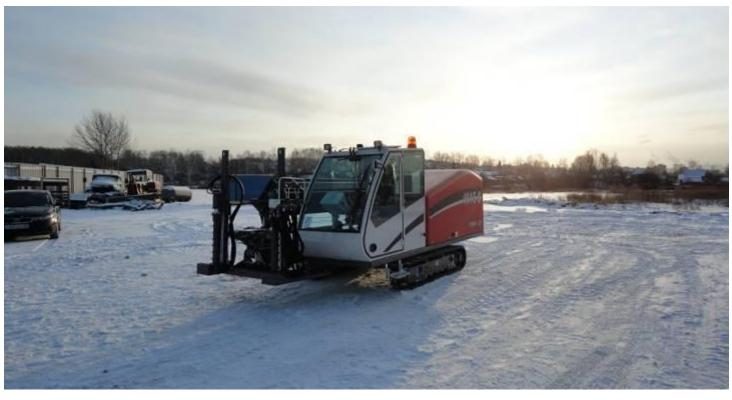
In the Russian city Beresovszky, which is 3 km (2 miles) away from Yekaterinburg, a new water line OD 110 mm (4") had to be laid trenchless over a distance of 220 m (726 ft). The first 150 m (495 ft) proceeded along the main road, the last 70 m (231 ft) were drilled through the forest.
