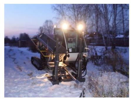
The TERRA-JET 4015 S in the drilling position. It is ready to start with the pilot bore.
