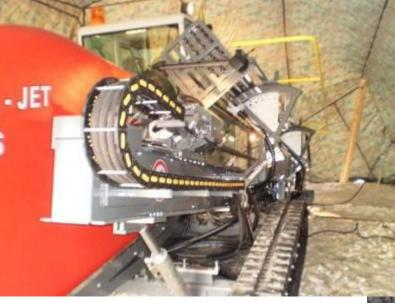
↑ The TERRA-JET 4015 S was operated inside a heated tent, to avoid the freezing of the Bentonite drilling fluid.
